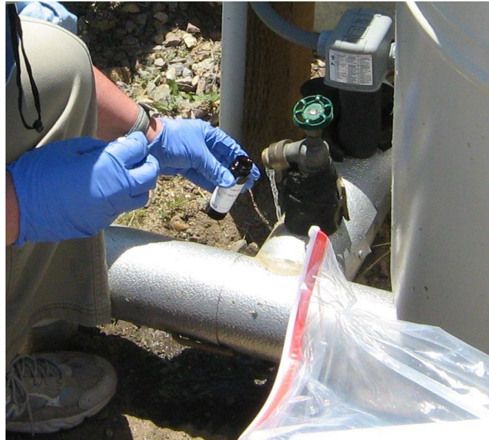
Figure 6. Individual collecting water sample from a spigot near the well head.
