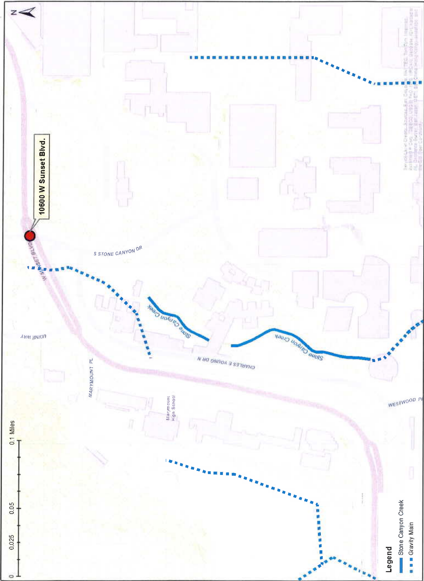
Fig.2 Stone Canyon Creek Relative to General Location of July 29, 2014 Westwood/Sunset Water Trunk Line Break.
