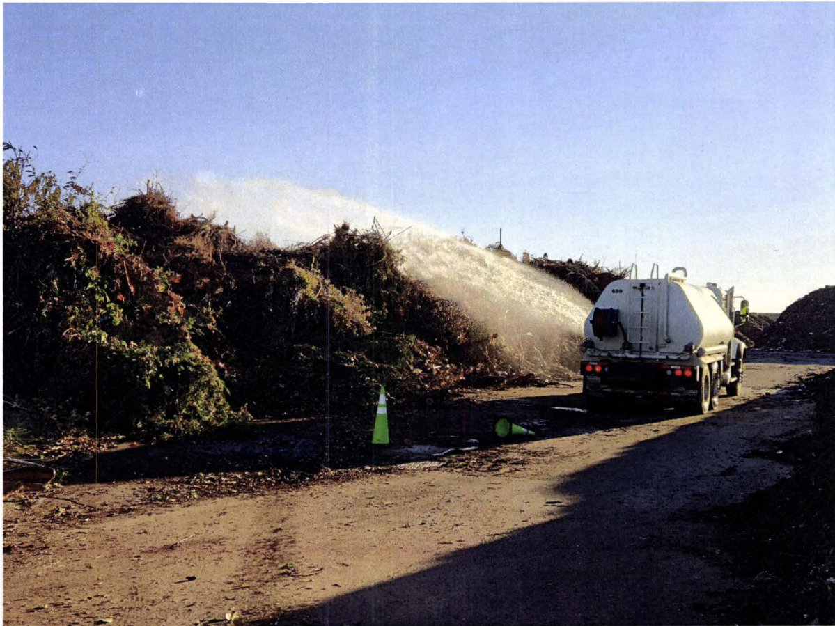
Figure 5: Water truck or fixed sprinklers will be used for recycled water addition. 10/3/22
