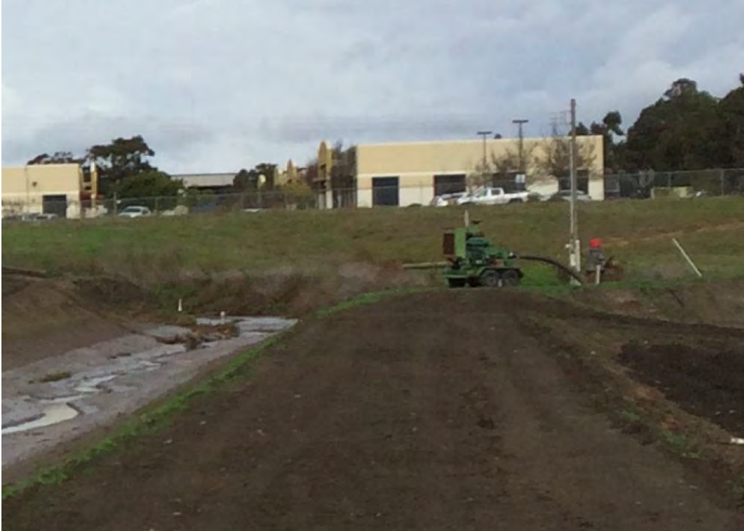
Figure 24. Photo taken of a large agricultural pump that discharges to Alisal Creek near monitoring station 309ALG. Photo taken by staff on January 9, 2019. The bank opposite the pump outlet was severely eroded.
