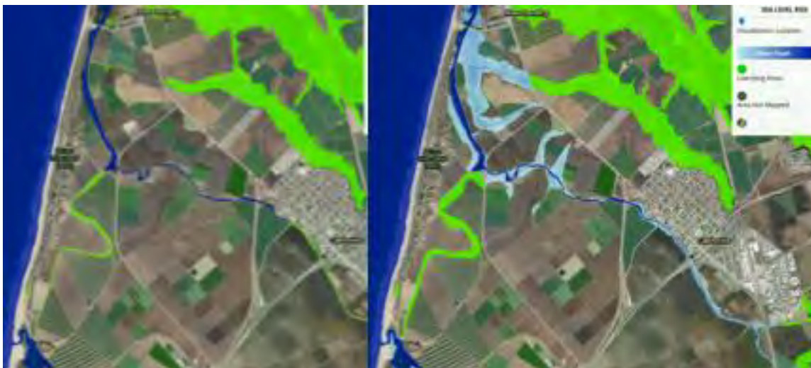
Figure 6. Map on left showing current sea level and second map on right showing 60 cm sea level rise near Castroville. (Source NOAA Sea Level Rise Viewer)
