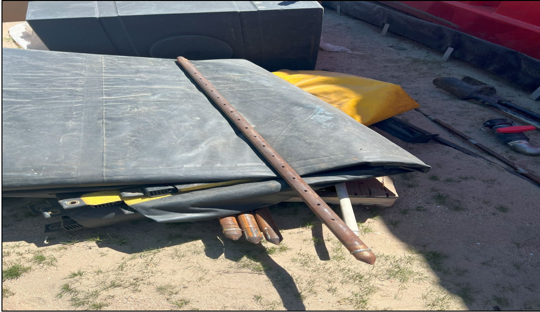
Photo 5.4: The 5-foot-long injection rod. EVO was injected into the subsurface at pressures as high as 150 pounds per square inch.
