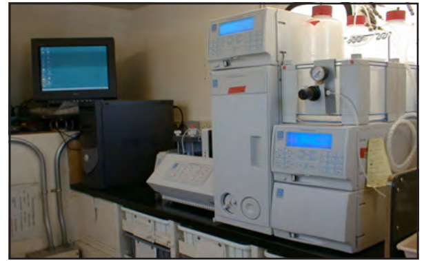
Figure 12. U.S. Geological Survey mobile laboratory and equipment to analyze chromium (VI).
