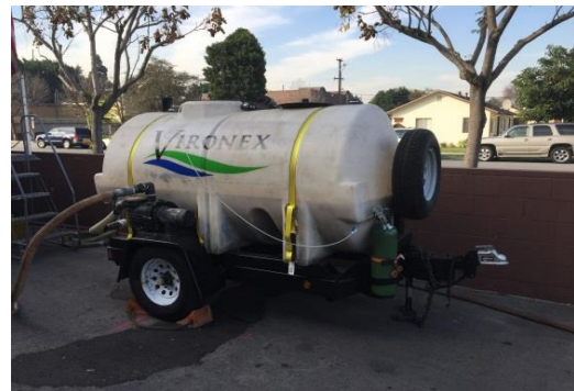
700 Gallon Water Trailer For Anoxic Water
