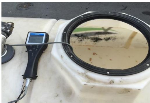
Testing Anoxic Water For DO
