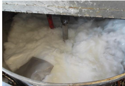
~138 Gallons of Water, ~14 Gallons of EOS-Pro and 4 Ounces of EOS-Pro Additive Mixed into a Solution
