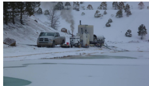
Emergency lime treatment of acidic mine drainage at Leviathan mine. Photo by: Chuck Curtis, Lahontan Regional Water Board.
