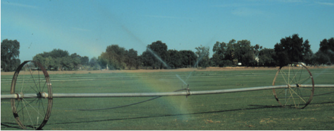
Wheel line irrigation of agricultural crops. Photo by: Dale Oliver, State Water Board.
