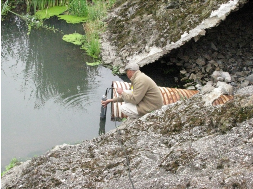
Photo 2. Water Board staff Habte Kifle monitoring the reservoir discharge for dissolved oxygen in 2010.
