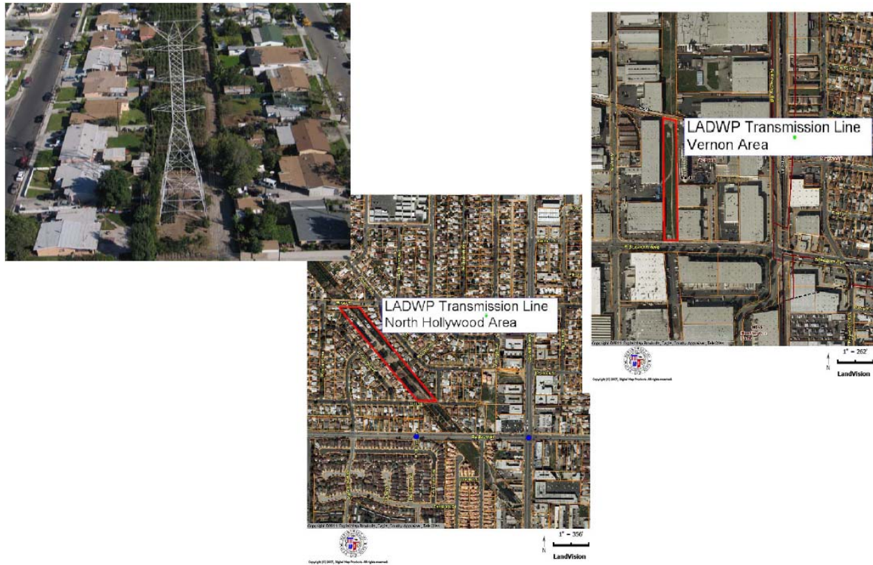
Figure 7 - Examples of how transmission growth is limited by residential and industrial growth along current right of ways
