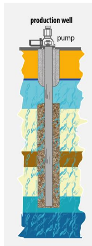
Figure 3-2: Groundwater Well Diagram
