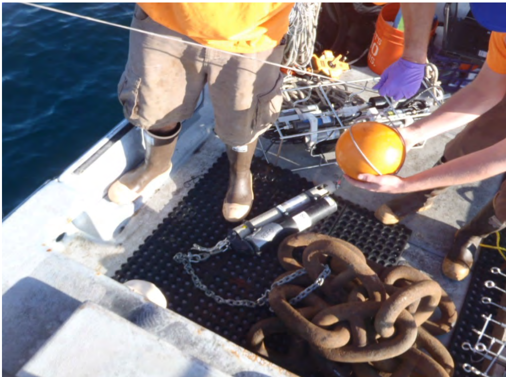
Photo 4: REF-01, finally, additional buoy, acoustic release, and anchor deployed
