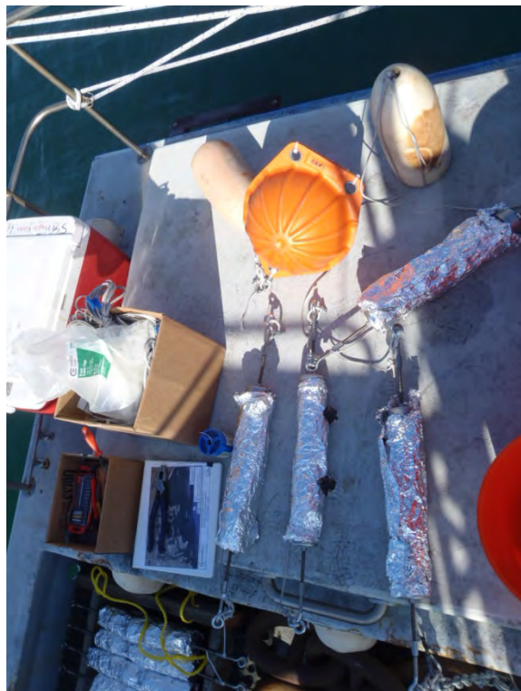
Photo 8: OB-01, mooring assembly: SPME assemblies (wrapped in foil) and buoys (anchor not shown on deck) prior to deployment
