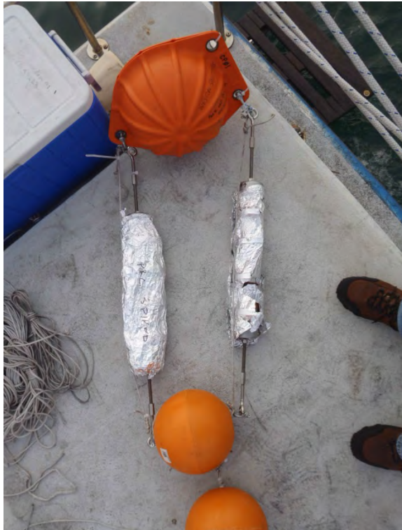
Photo 25: CP-01, top to bottom of mooring assembly– hard hat buoy, then SPME assemblies, then buoys (continued on next photo)
