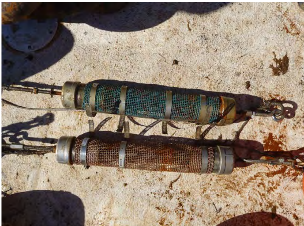
Photo 6: OB-01 Bottom depth (PRC on top and primary sample below in photo)
