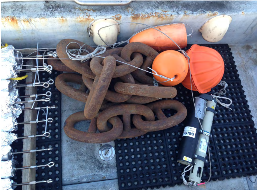
Photo 1: REF-01, mooring assembly: buoys, SPME assemblies (on rack), and anchor prior to deployment
