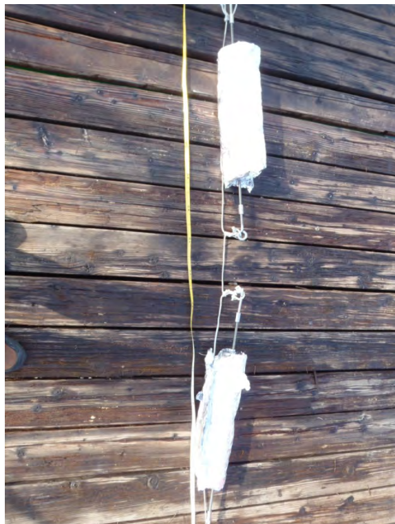
Photo 34: FH-01, top to bottom of mooring assembly –SPME assemblies (continued on next photo)
