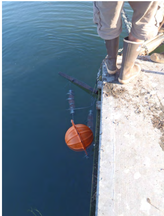
Photo 24: LARE-01, SPME assemblies after parallel reconfiguration
