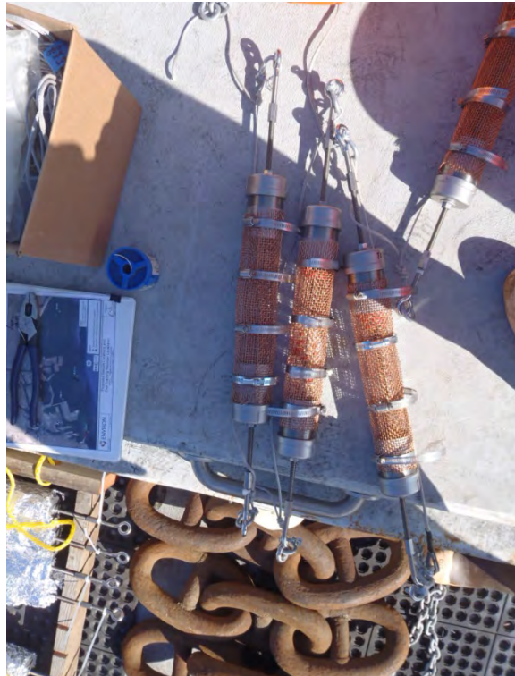
Photo 9: OB-01, SPME assemblies (without foil, as deployed) prior to deployment
