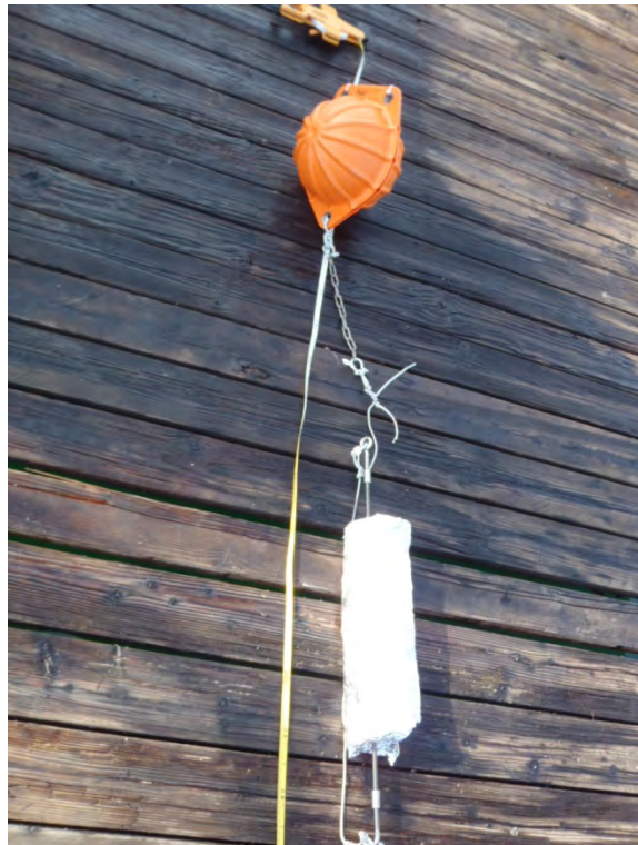
Photo 33: FH-01, top to bottom of mooring assembly –hard hat buoy, then SPME assemblies (continued on next photo)
