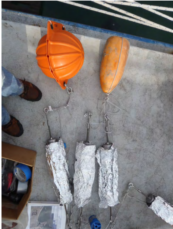
Photo 43: CS-01, mooring assembly prior to deployment
