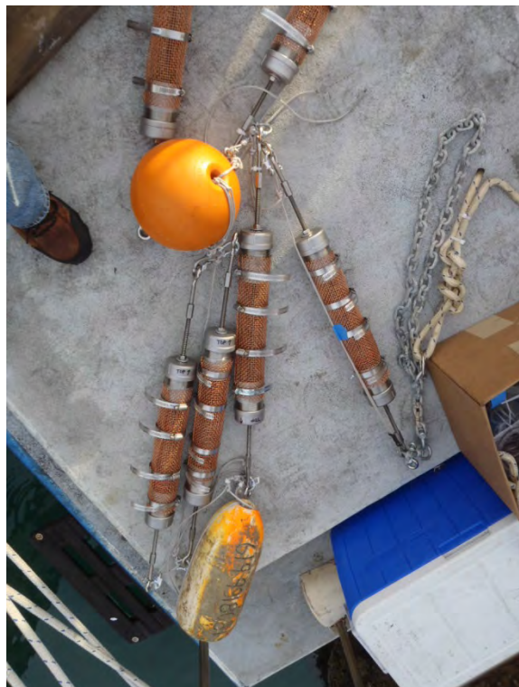
Photo 46: IB-01, top to bottom of mooring assembly prior to deployment (anchor not shown)
