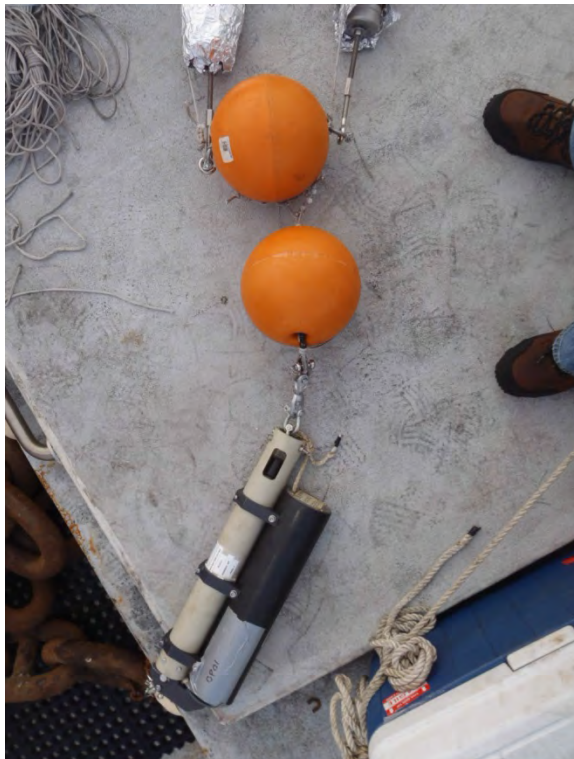
Photo 26: CP-01, top to bottom of mooring assembly –buoys, then acoustic release (continued on next photo)
