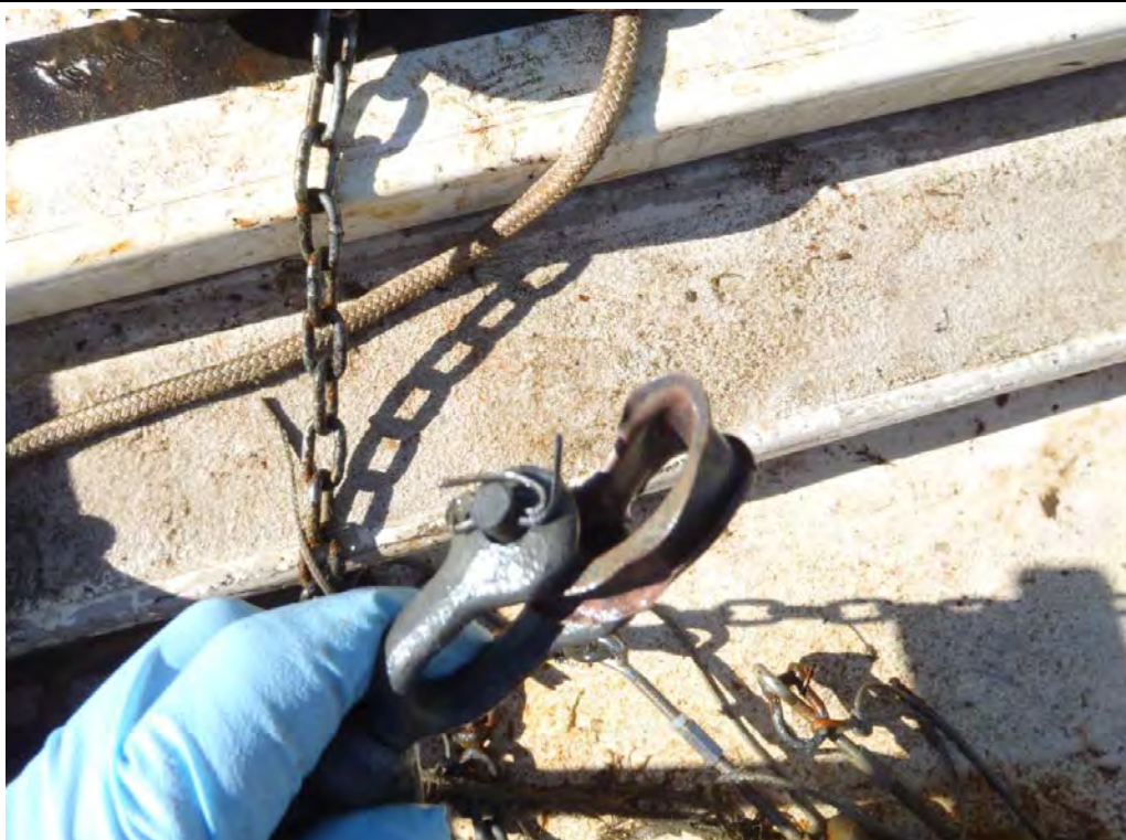
Photo 10: SP-01, thimble bent
