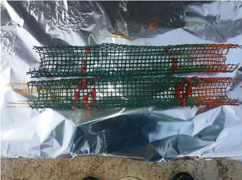
Photo 23: IA-01, Inner housing for fibers (PRC on top and primary sample below in photo)
