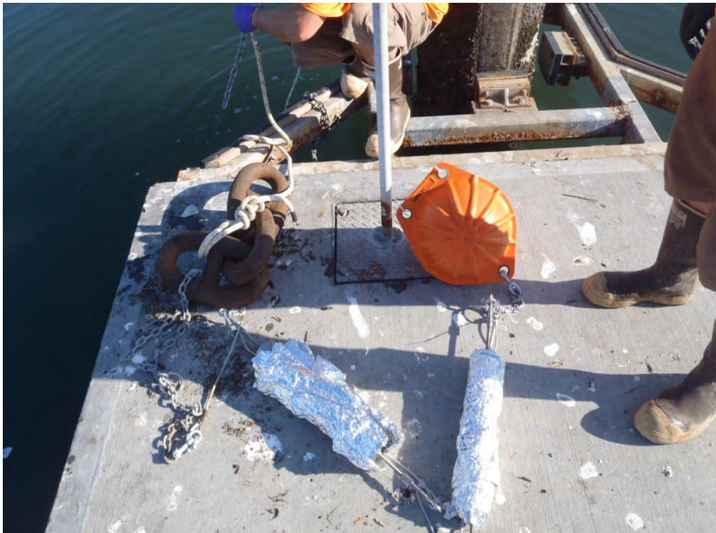
Photo 23: LARE-01, tie off to dock (photo taken prior to parallel reconfiguration for SPME assemblies)
