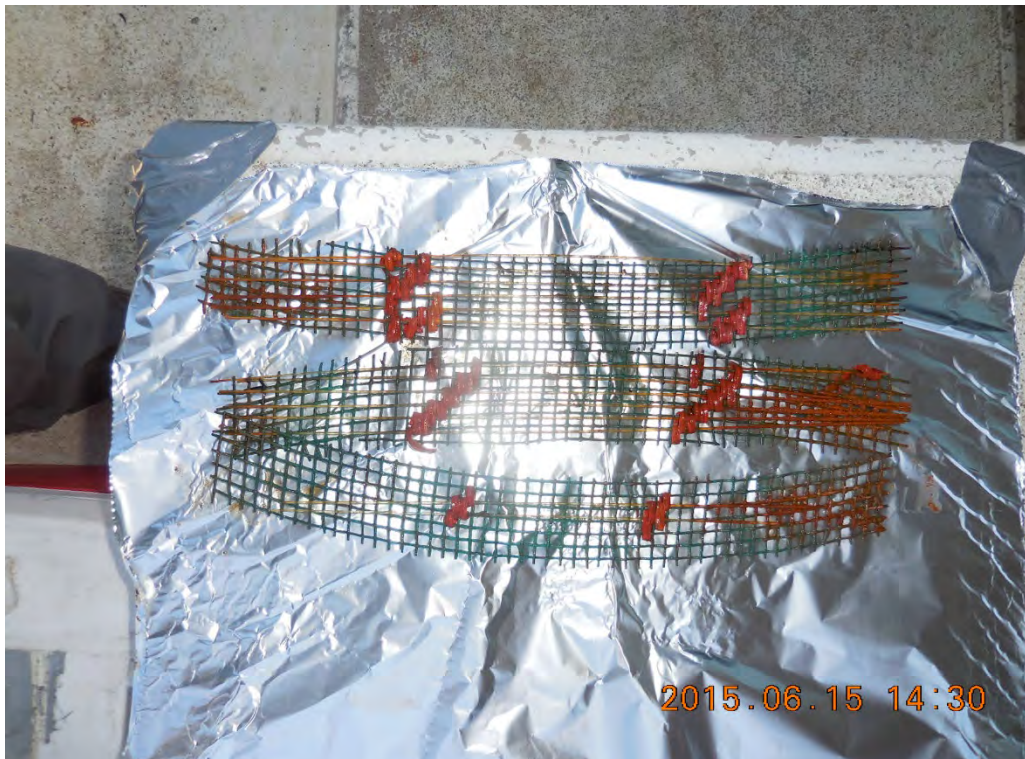
Photo 8: IB-01 Mid-depth Primary and PRC SPMEs
