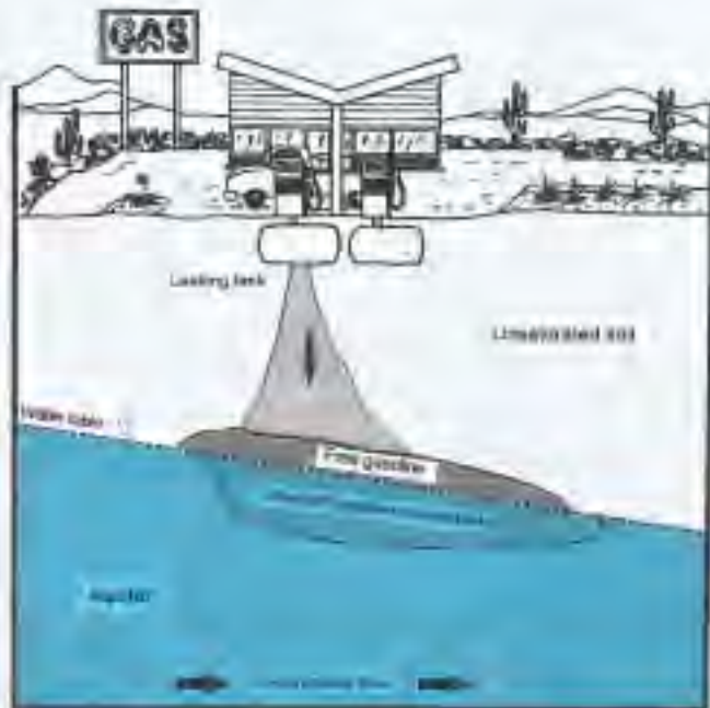
Figure 4-9. Leaking underground storage tank. This diagram illustrates how contamination of the vadose zone and pollution of ground water can result from leaks of gasoline from an underground storage tank (Adapted from Fetter, 1988).
