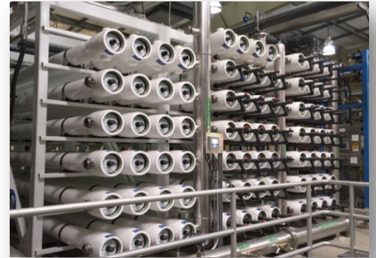
Reverse osmosis systems to remove salt from pumped groundwater. Photo Credit: Yucaipa Valley Water District
