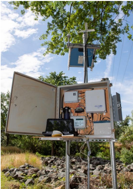
Figure 3. A view of the station house for the newly installed North Honcut Stream Gage on Honcut Creek in Butte County.
