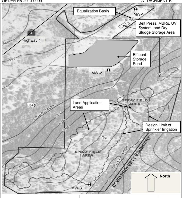
Drawing Reference: Figure 4, Geologic Map Workplan for Installation of Groundwater **Monitor Wells** May 2012, Condor Earth Technologies, Inc.
