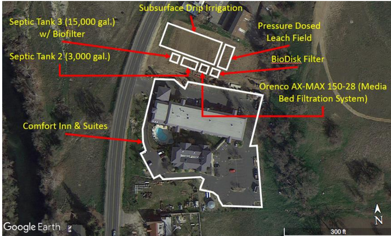
ATTACHMENT A – SITE MAP NOTICE OF APPLICABILITY 2014-0153-DWQ-R5314 FOR BSK INVESTMENT, LLC; COMFORT INN & SUITES SEQUOIA KINGS CANYON ONSITE WASTEWATER TREATMENT SYSTEM TULARE COUNTY
