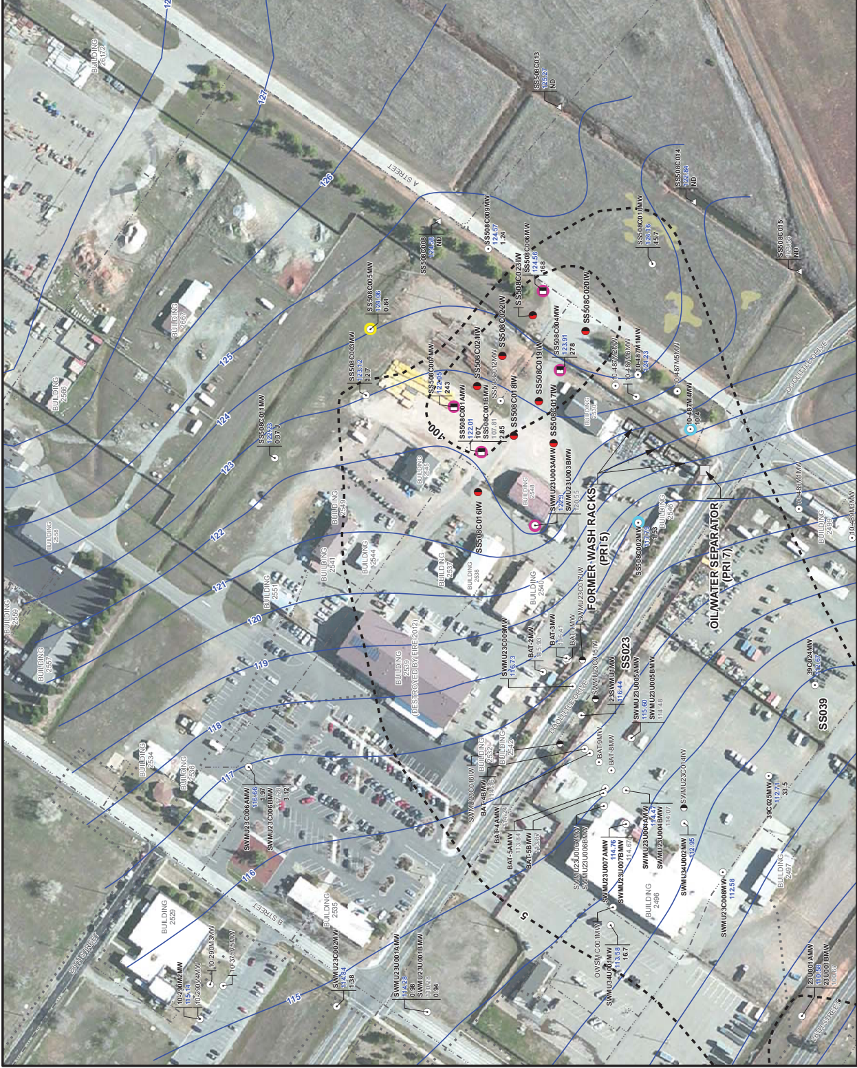
FIGURE 5-2 CG041-508 PROPOSED ERD INJECTION WELL LOCATIONS CG041-508 STATEMENT OF BASIS/CORRECTIVE MEASURES IMPLEMENTATION WORK PLAN FOR GROUNDWATER BEALE AIR FORCE BASE, CALIFORNIA
