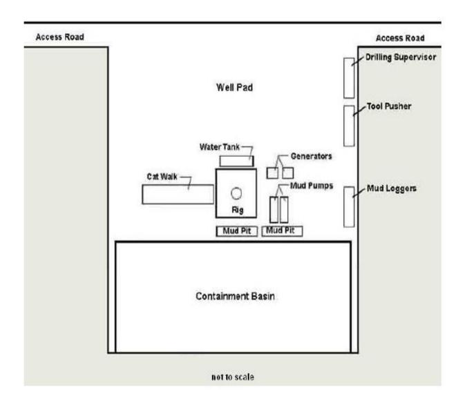
Figure 5: Typical Well Pad Layout Diagram
