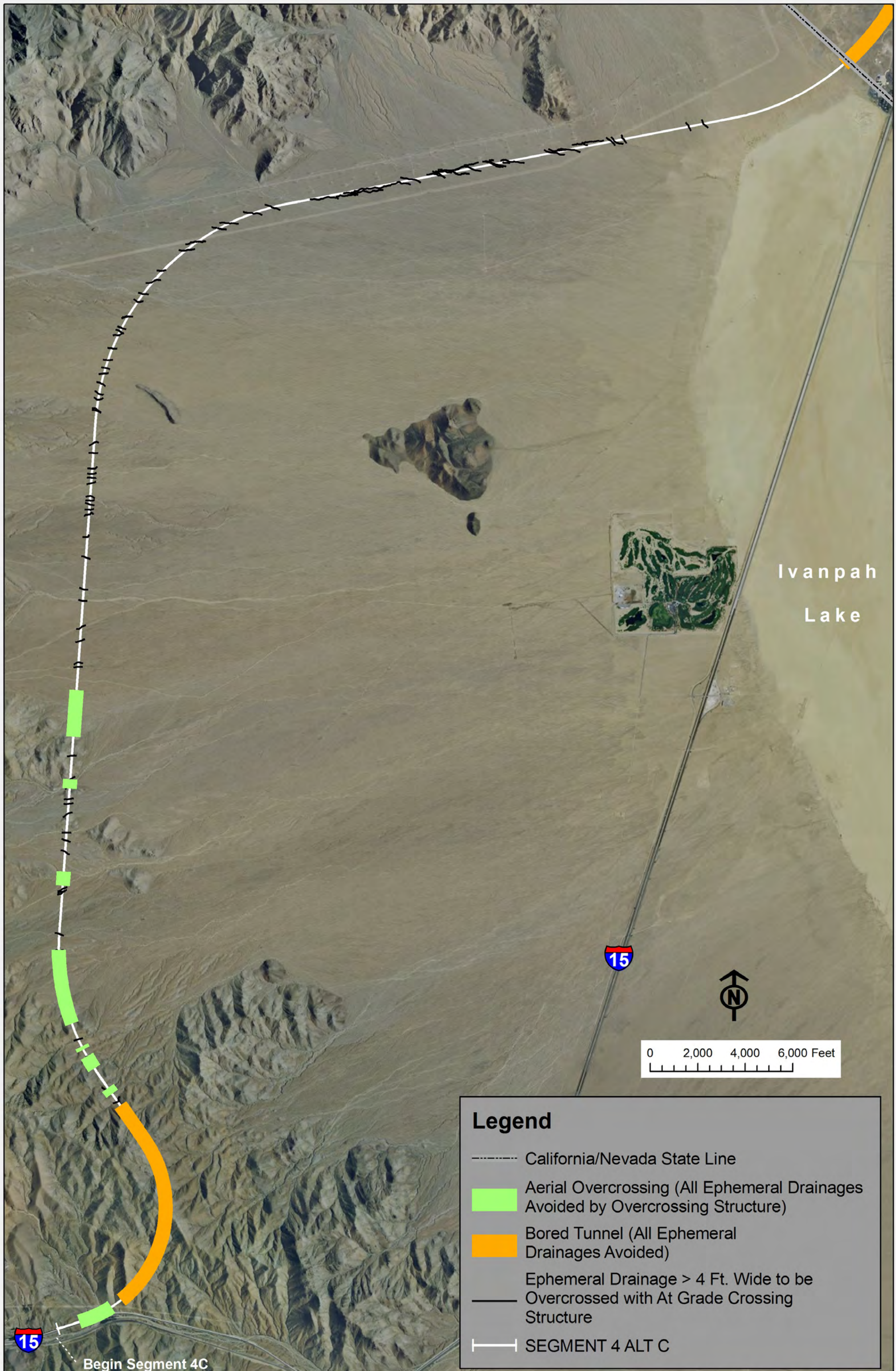
Figure 2. Preliminary Location of Aerial and At-Grade Crossings Within the California Portion of Alternative 4C, DesertXpress Project
