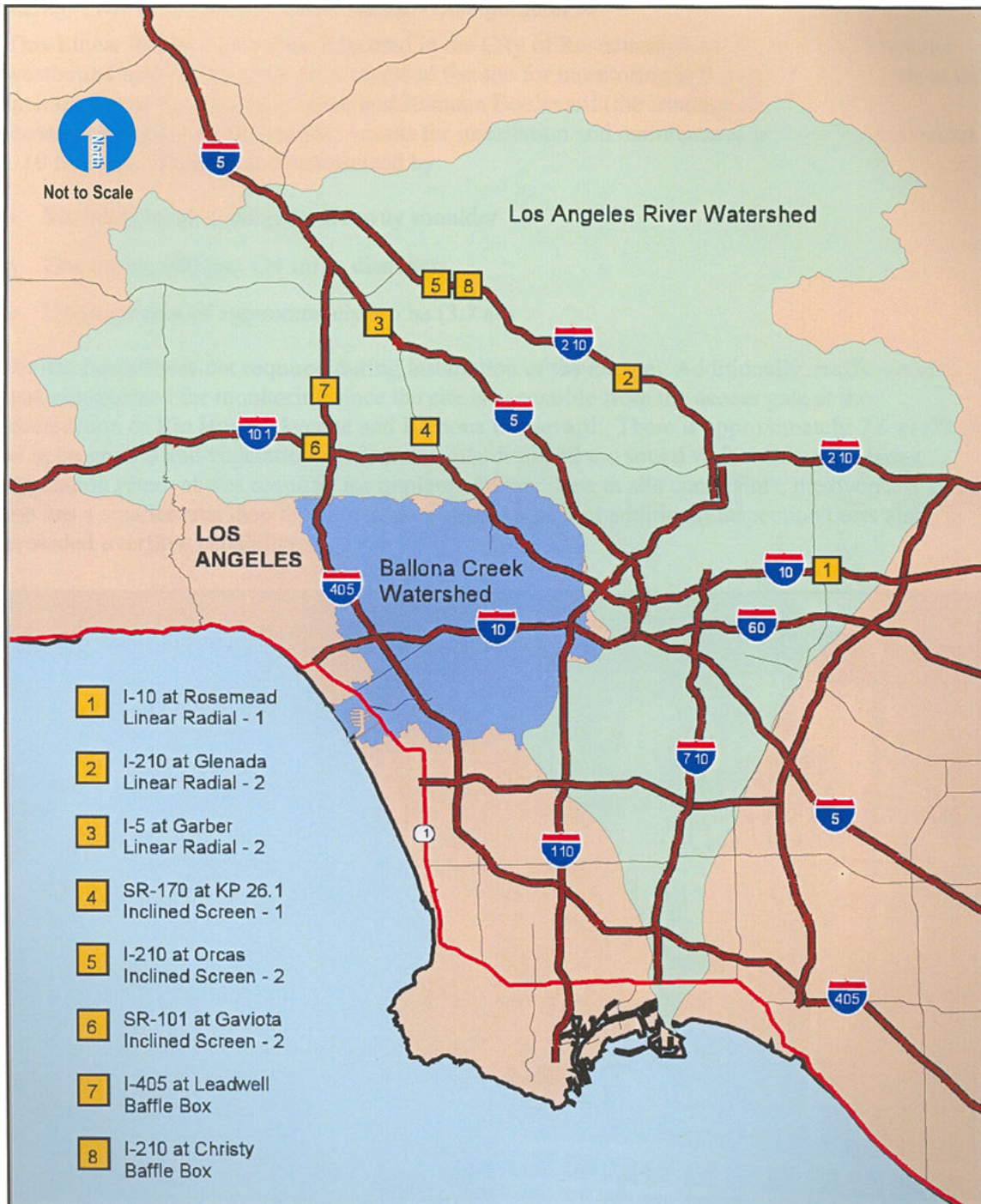
Figure 8-4: GSRDs Located in the Los Angeles River Watershed as of October, 2003. (Source Caltrans, 2003b)
