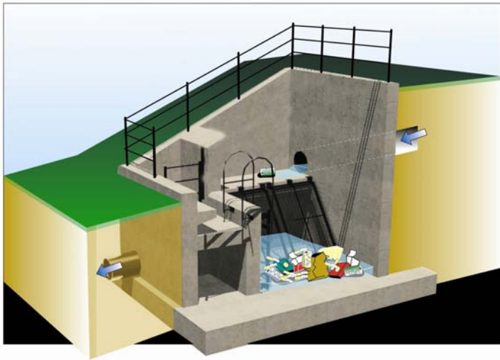
Figure 5-11. Inclined Screen Device – Type 2
