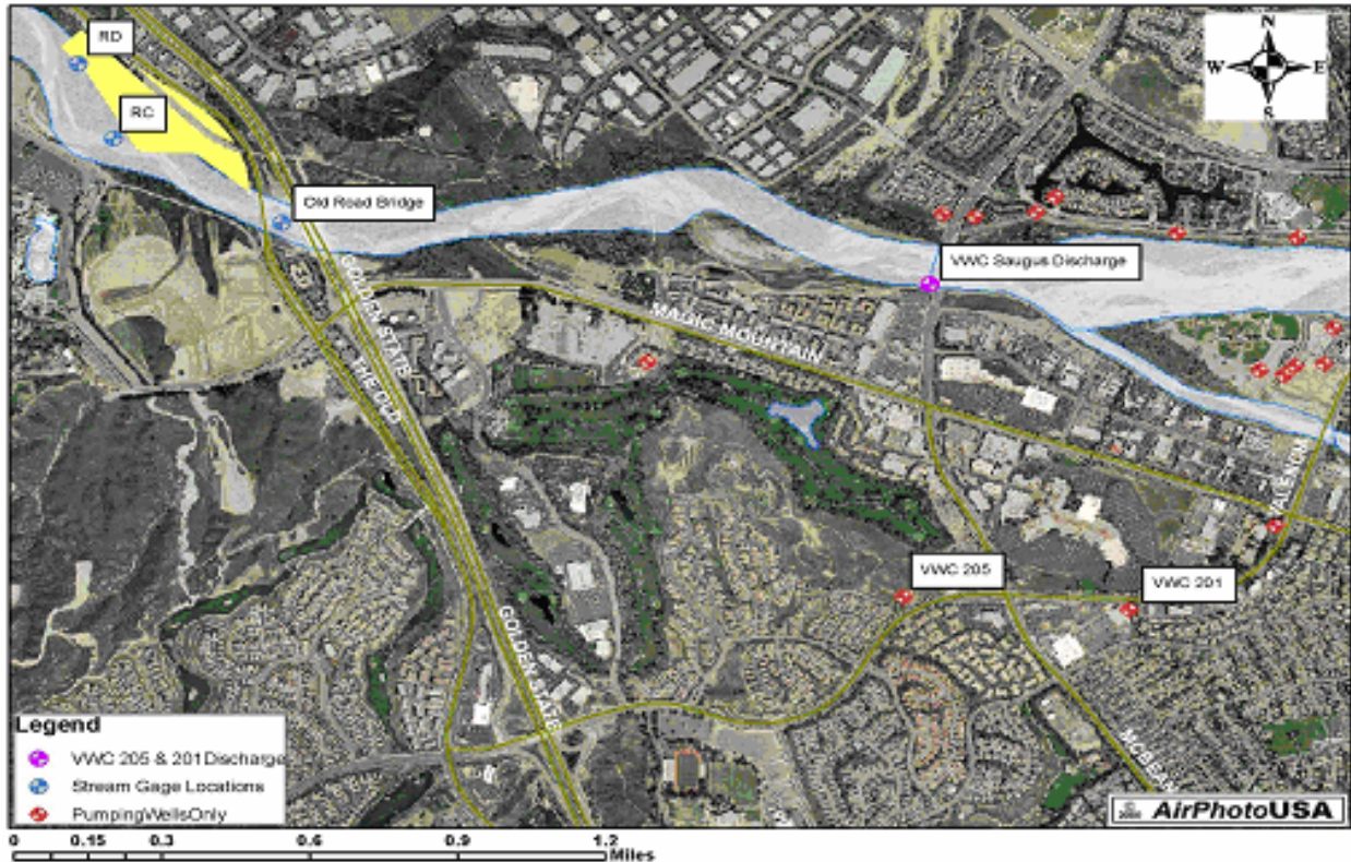
Figure 7. Existing Saugus Aquifer Wells (VW-201/205) and Discharge Point of Supplemental Water
