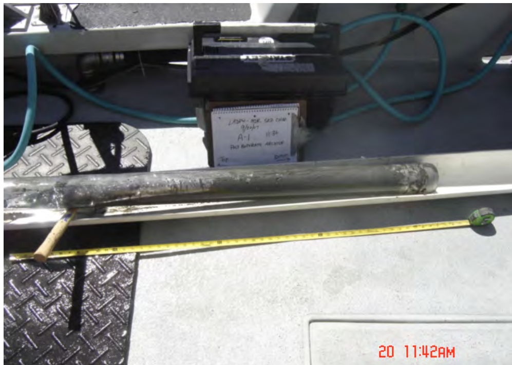
Figure 5. Core tube archive sample collected using vibracore grab sampler.
