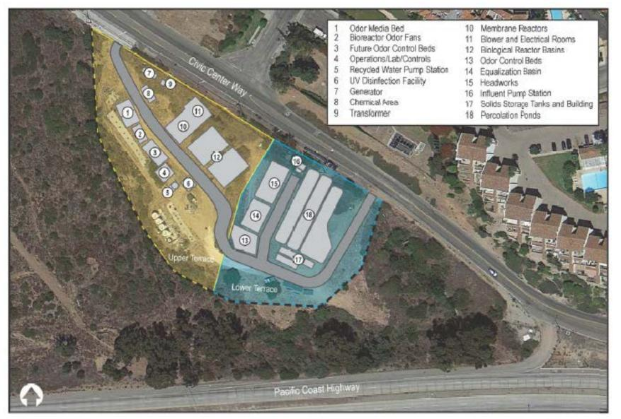
Figure 3 – Layouts of Malibu Civic Center Wastewater Treatment Facility
