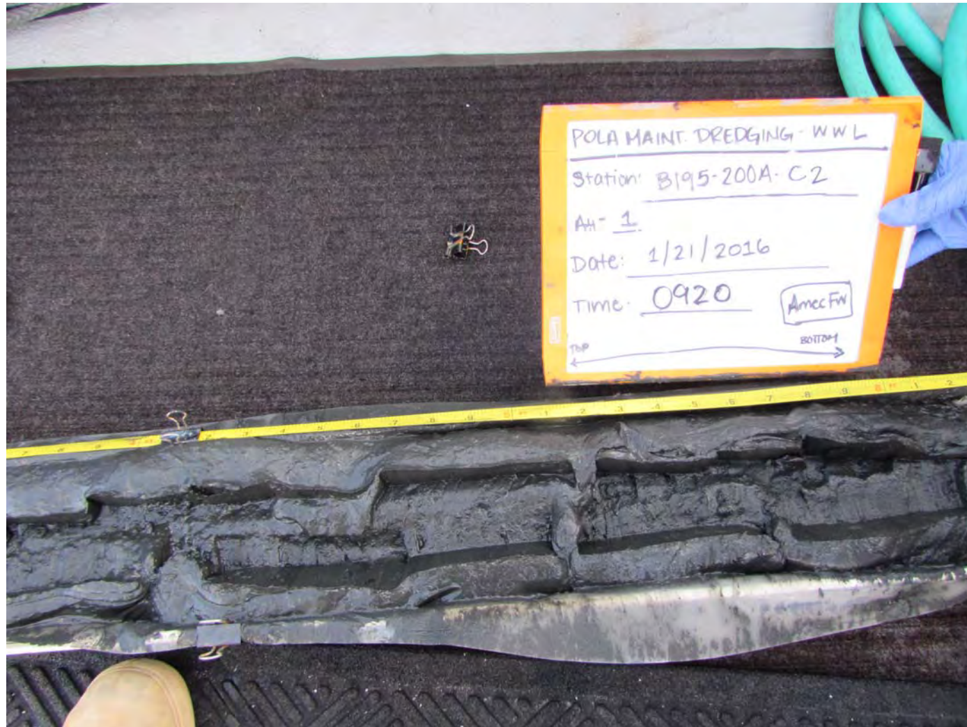
Location: POLA Berths 195-200A Sample ID: B195-200A-C2 Attempt #: 1 Core Length: 4.0 - 6.3 ft. Sample Date & Time: 01/21/2016 0920
