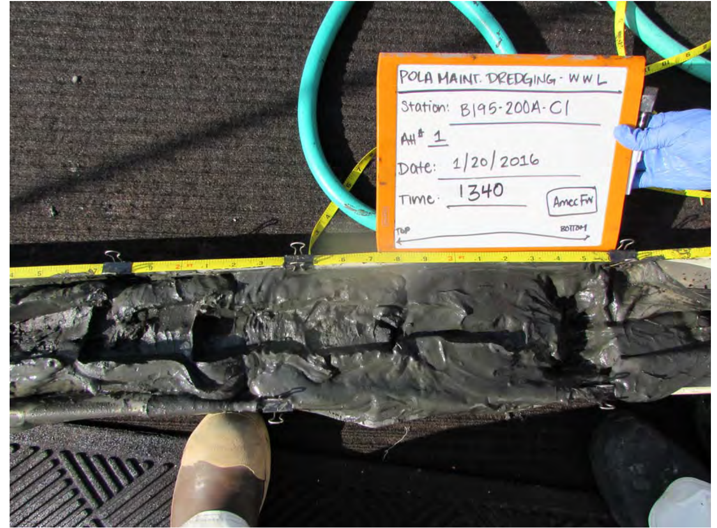
Location: POLA Berths 195-200A Sample ID: B195-200A-C1 Attempt #: 1 Core Length: 2.0 - 3.4 ft. Sample Date & Time: 01/20/2016 1340
