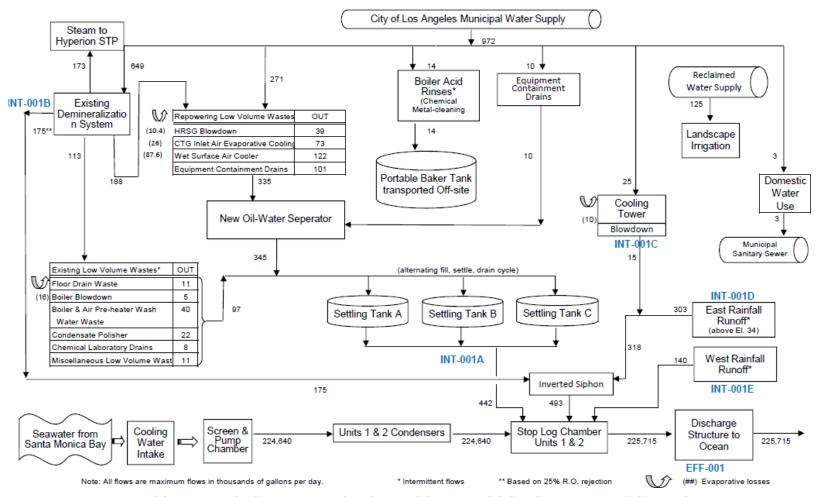
SCHEMATIC of WATER FLOW for the SCATTERGOOD GENERATING STATION
