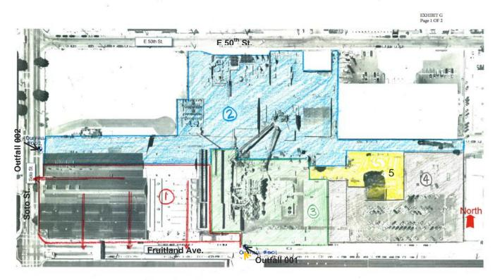
Plant Site Drainage Diagram Upon Completion of the Outfall 002 Drainage Improvement Project:
