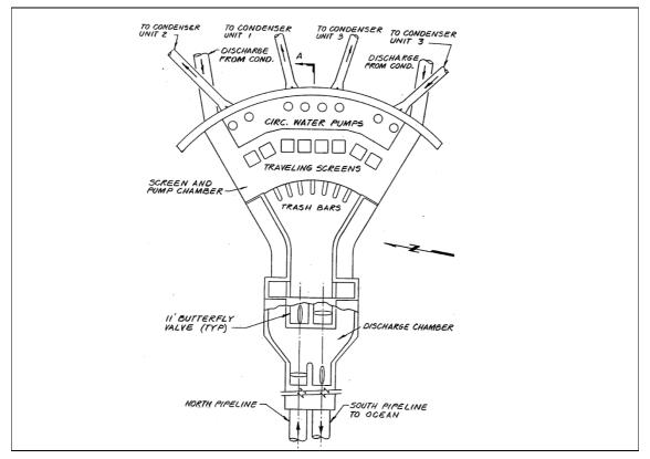
Figure 3.2-3. Plan view of the SGS onshore intake structure.
