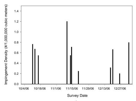
Figure 5.5-91. Concentration (# / 1,000,000 m<sup>3</sup> [264.172 million gal]) of spiny lobster collected in SGS VCS normal flow impingement samples (Oct. 4, 2006 – Jan. 3,
