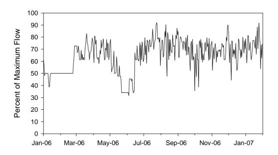
Figure 3.2-5. Daily cooling water flow volumes at the SGS from January 2006 to February 2007. (Maximum = 1,874,938 m<sup>3</sup> per day, or 495.360 mgd)
