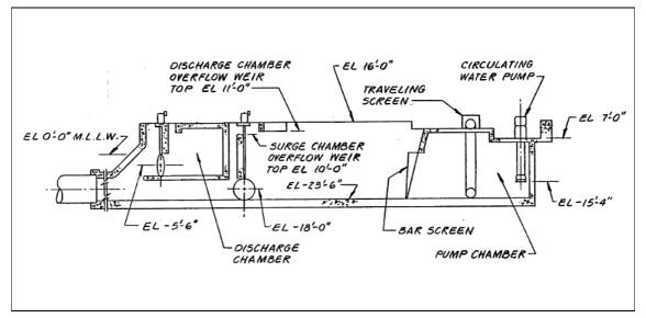
Figure 3.2-4. Section view of the SGS onshore intake structure.
