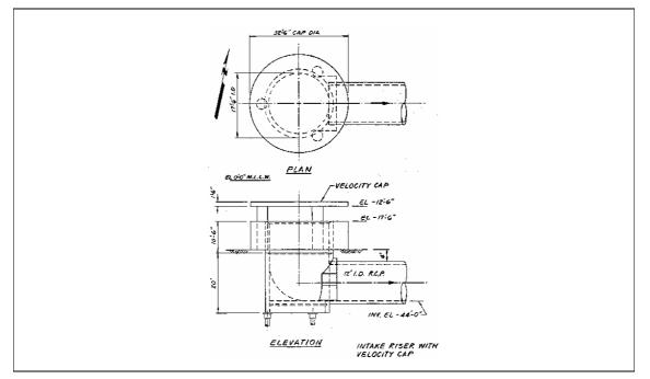
Figure 3.2-2. Detail of the SGS offshore intake riser and velocity cap.
