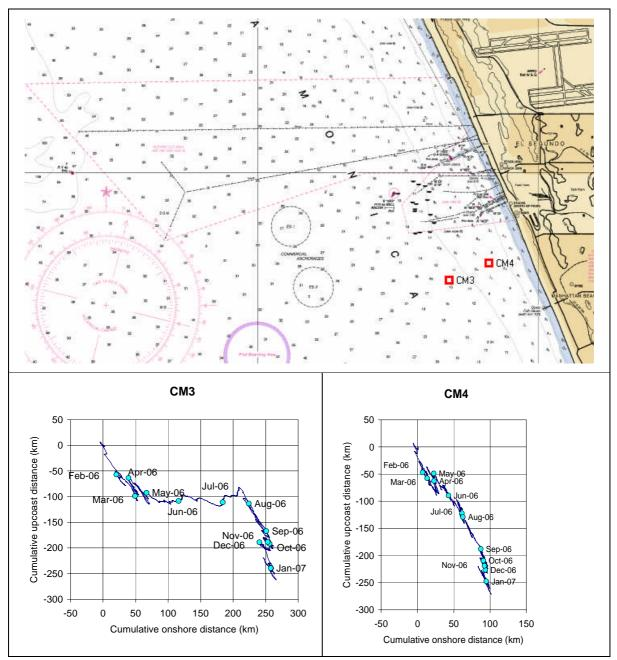
Figure 3.3-5. Net displacement at current meter stations CM 3 and CM 4 from January 2006 to January 2007.
