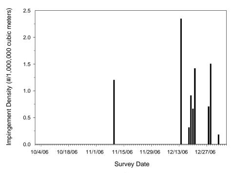
Figure 5.5-62. Concentration (# / 1,000,000 m<sup>3</sup> [264.172 million gal]) of Pacific rock crab collected in SGS VCS normal flow impingement samples (Oct. 4, 2006 – Jan. 3, 2007).
