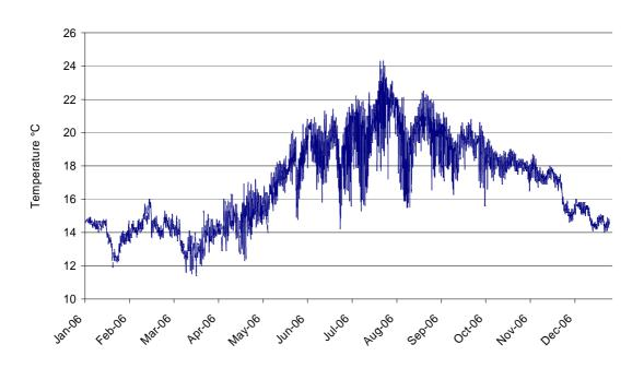
Figure 3.3-2. Hourly surface water temperatures at NOAA Station 9410840 at Santa Monica Pier, California from January through December, 2006.
