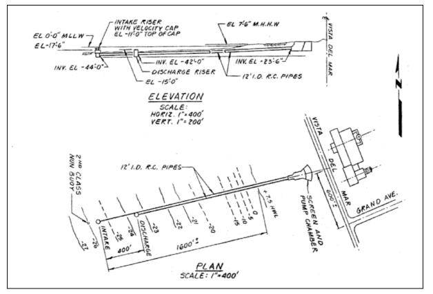
Figure 3.2-1. Plan view and elevation of the SGS offshore intake system.
