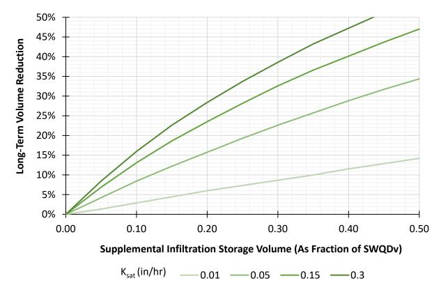
Figure 4: Volume Reduction Provided by a Supplemental Infiltration Compartment
