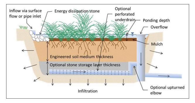
Figure 1: Cross sections of typical biofiltration system
