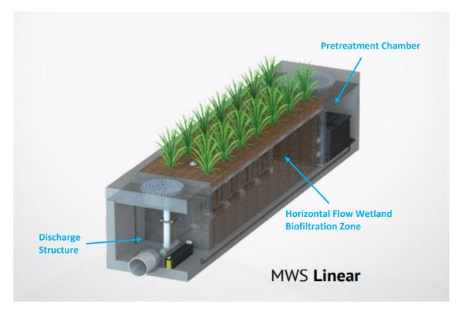
**Figure 2: Typical MWS Linear Configuration**
