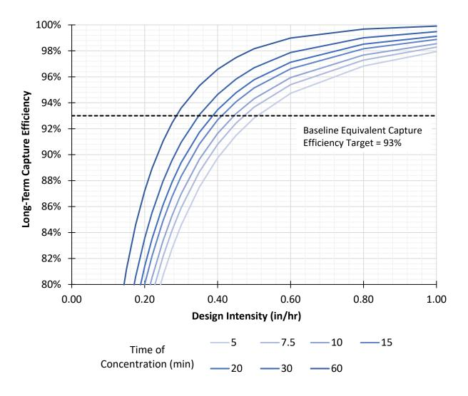
Figure 3: MWS Long-Term Capture Efficiency based on Design Intensity and Time of Concentration
