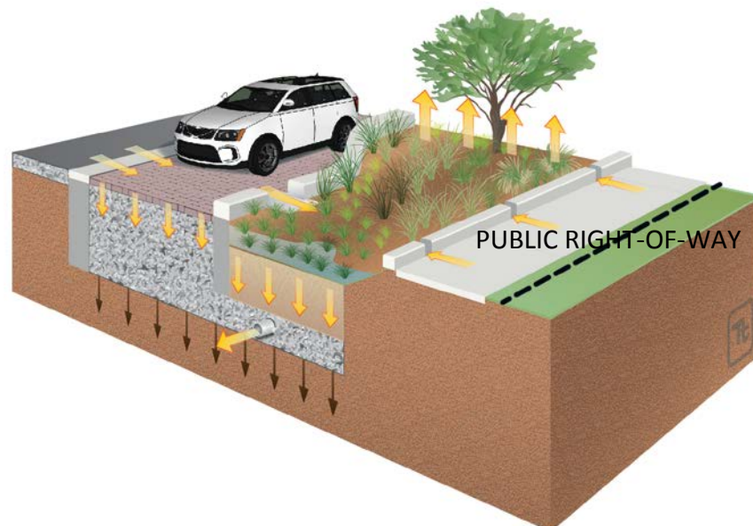
Figure E-8 Typical Distributed Green Street Schematic (arrows indicate water pathways)
