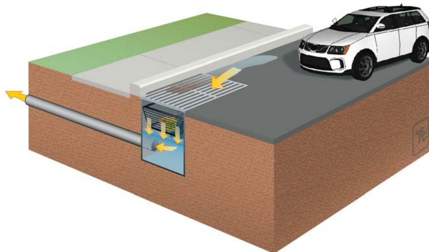
Figure D-13 Typical Distributed Source Control Structural BMP Schematic (arrows indicate water pathways)
