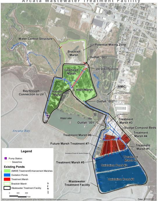
Proposed WWTP Flow Configuration Arcata Wastewater Treatment Facility
