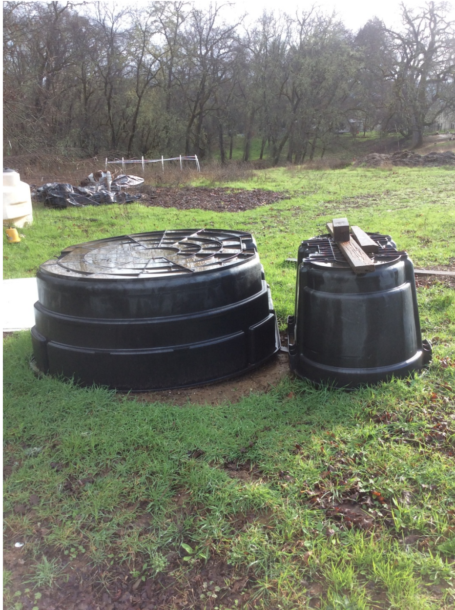
Picture 3: This is a photograph of the fertilizer mixing station facing east. The mixing station consists of a 300 gal. tank and a 100 gal. tank. Photo date 2-18-16.
