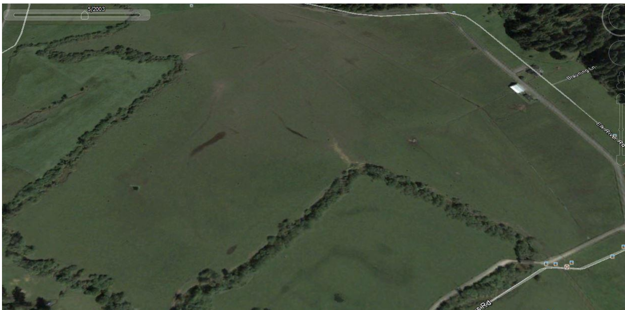
Figure 9. Section of the Elk River floodplain in the affected reach with some residual channel features in the floodplain. The five right-angle bends in this image show the extent to which the main channel has been altered by human activities, and the presence of these sharp bends
