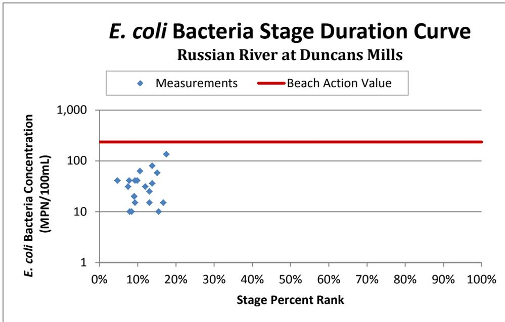
Figure 37. *E. coli* Bacteria Stage Duration Curve for measurements made in the Russian River at Duncans Mills
