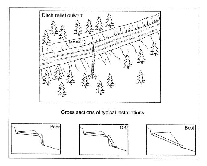
Figure X-19. Typical ditch relief culvert installation.
