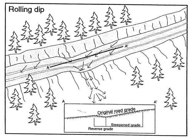
Note: Rolling dips must drain the road surface and be driveable for the expected traffic.
