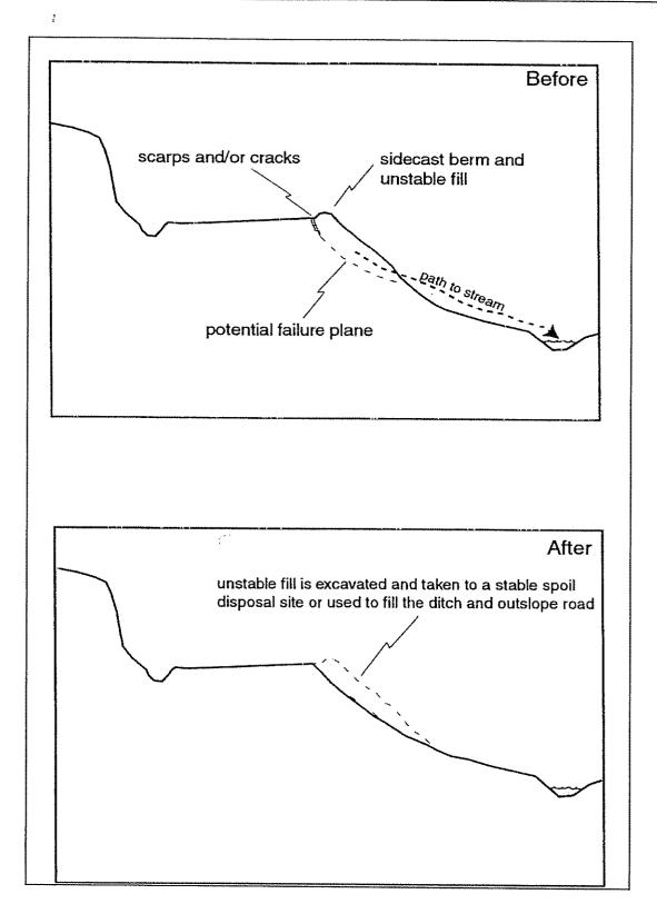
Figure X-17. Removal of unstable sidecast materials.
