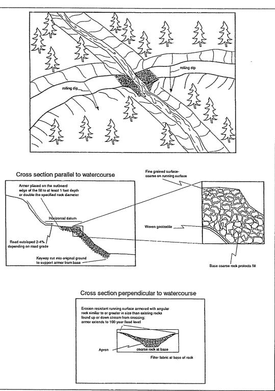
Note: Where geotextile fabric may interfere with passage of amphibians in any Class 2 or 3 crossing, bury geotextile fabric with at least 6 inches of rock. Do not use geotextile fabric in fish-bearing streams.
