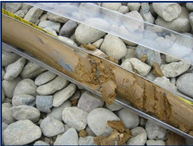
Figure 1 – DPT Core Showing ZVI Distribution
