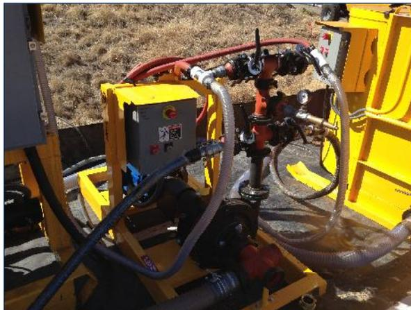
Figure 2 – Shear pump used to create a uniform guar mixture to adequately suspend ZVI
