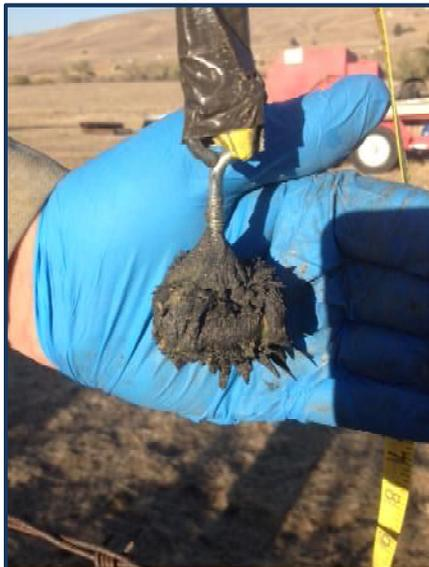
Figure 1 – Magnet recovering ZVI from target monitoring well 15' from injection location
