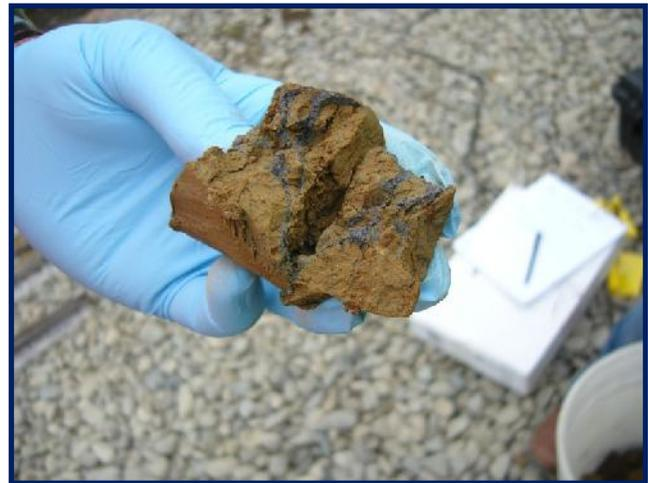
Figure 2 – DPT Core Showing ZVI Throughout Core
