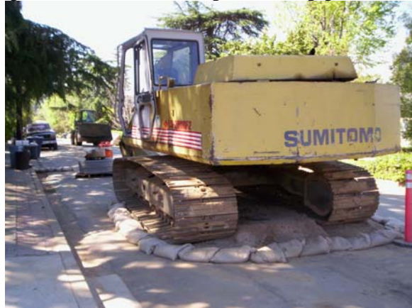
Photo 13. Leaking equipment requiring maintenance. Photo 14. Secondary containment around vehicle.
