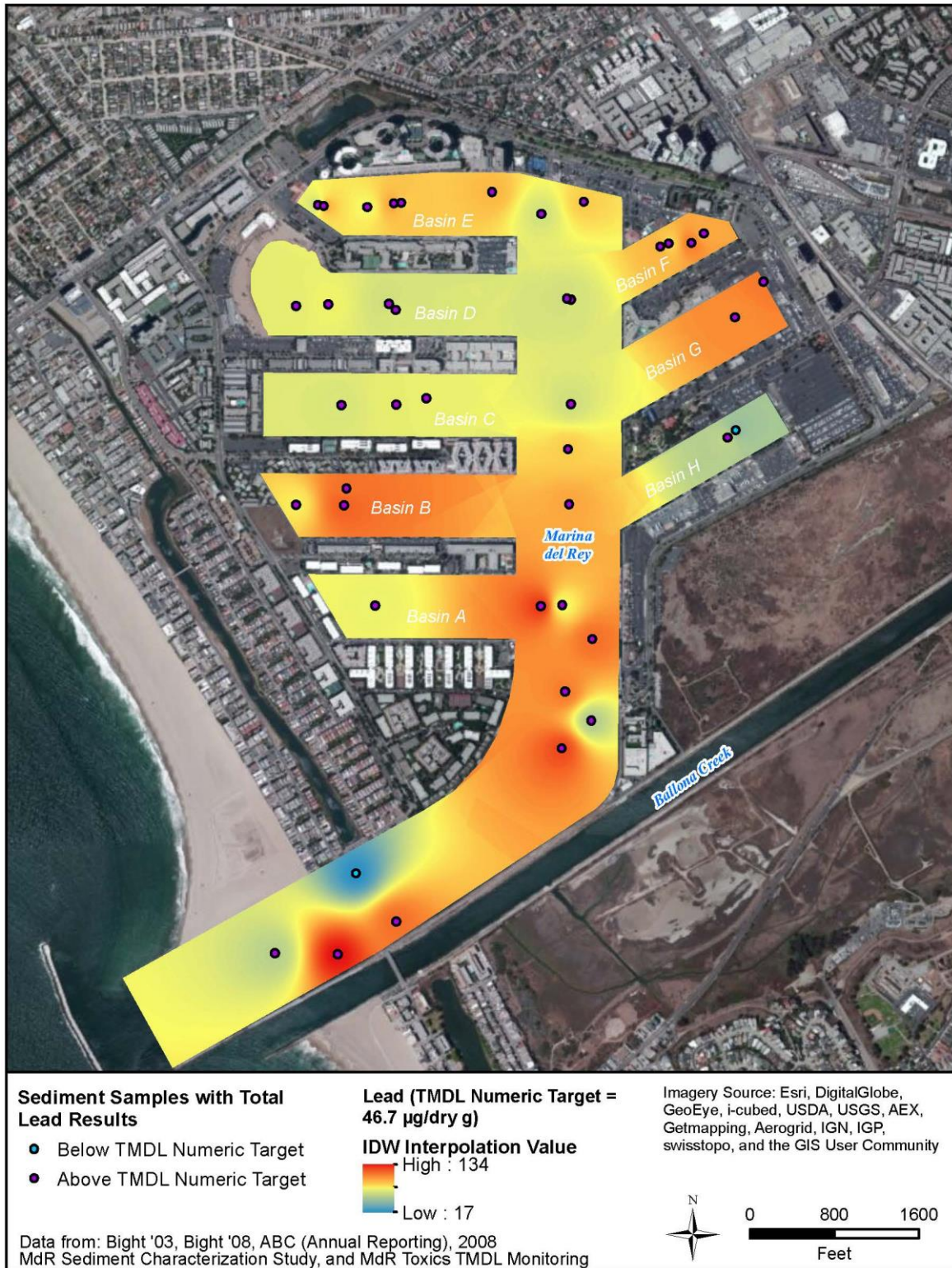
Figure 5. Marina del Rey Harbor Sediment Lead Concentrations, 2002 to 2013
