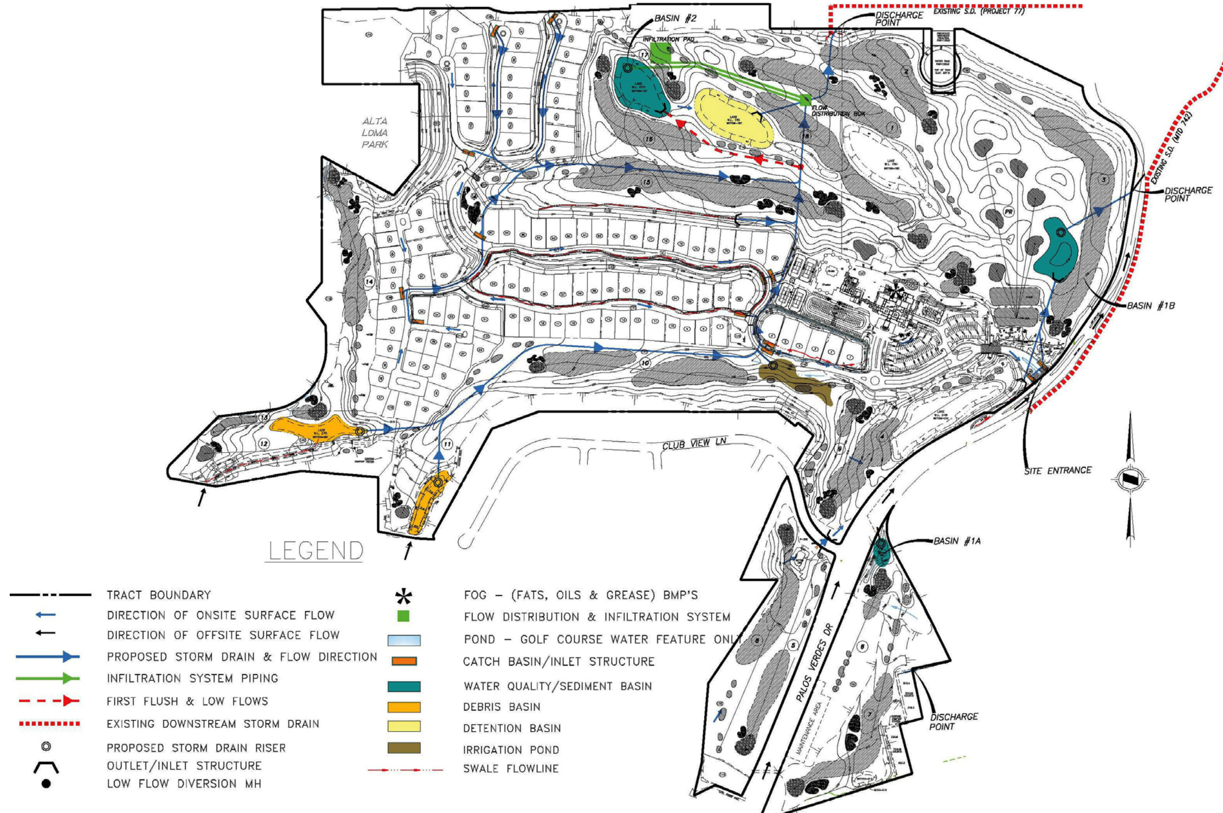
Figure 3-9: Chandler Quarry Project Drainage and Water Quality Concept Plan Source: Hunsaker and Associates. Water Quality Mitigation Plan. June 16, 2010.
