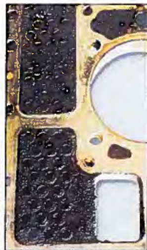
Heavily carbonized valves and cooler tubes of a starting air compressor
