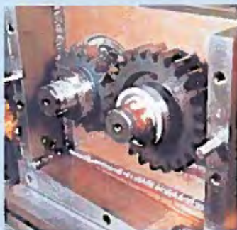
Left: An FZG test rig used to assess the load-carrying capacity of slow-speed engine system oils.
