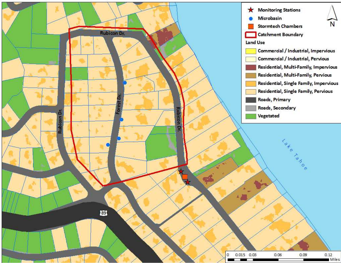
Figure 9: Rubicon monitoring site, including monitoring station locations, Stormtech chambers location, catchment boundary, and land use distribution.
