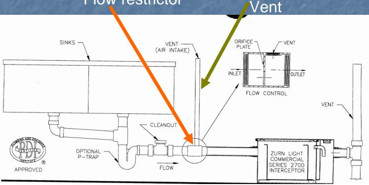
**GREASE TRAPS** "Under the Sink" Units Sizes – most common \* 20gpm/40 lb. capacity 10 gpm / 20 lb capacity trap is City of Clarksville minimum acceptable 15 gpm / 30 lb capacity size 20 gpm / 40 lb capacity\* 25 gpm / 50 lb capacity 35 gpm / 70 lb capacity Most floor traps will have sizing (flow rate and capacity) on the 50 gpm / 100 lb capacity under -side of the top cover
