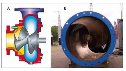
Figure 3. (A) Cut away diagram of a screw centrifugal impeller (Source: Hidrostal) and (B) impeller of Bedford pumps SAF.90.05.12 (Source: Spierts and Vis 2012).
