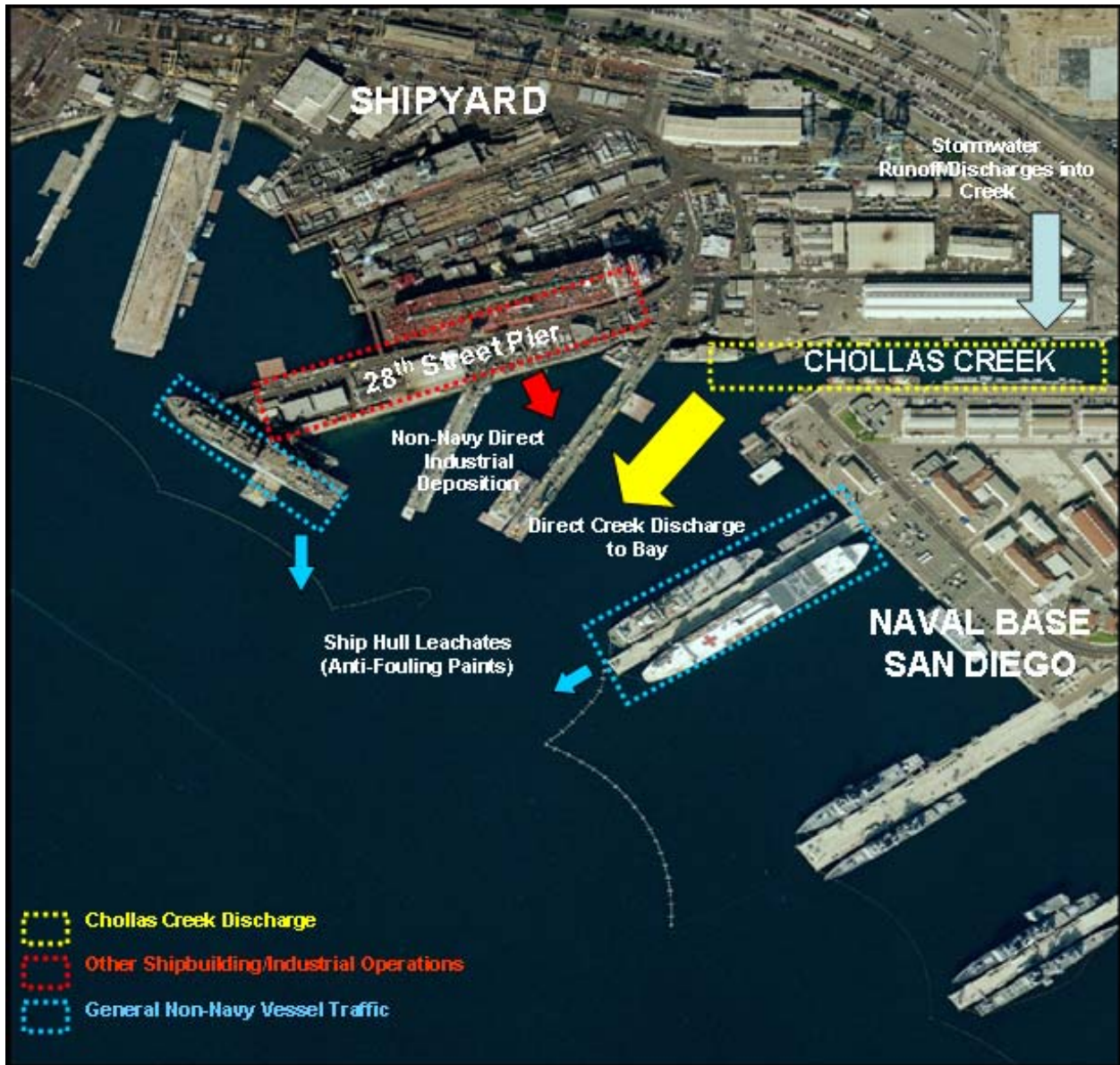
Figure 7. Conceptual site model of contaminant input and fate for potential source Pathway 2 at the Chollas Creek mouth area.
