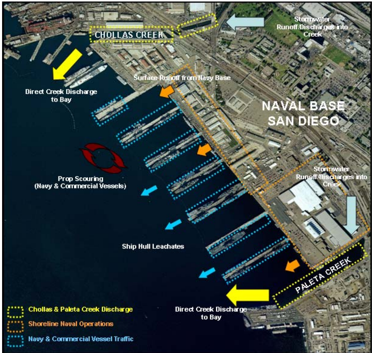
Figure 13. Conceptual site model of contaminant input and fate for potential source Pathway 3 at the Naval Base San Diego area.
