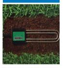
Soil moisture sensors are placed below ground in the root zones of lawns and landscapes to determine if and how long to water. Sensor-based products are available as stand-alone controllers or add-on devices to existing controllers. They have been shown to reduce outdoor water use by up to 70% without sacrificing the quality or health of your landscape.
