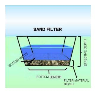
The filter discharge is calculated using the equation Q = K\*I\*A, where Q is the discharge in cubic feet per second (cfs). K equals the hydraulic conductivity (inches per hour). For sand filters K = 1.0 in/hr. Sand is the default medium. If another filtration material is used then the design engineer should enter the appropriate K value supported by documentation and approval by the reviewing authority.
