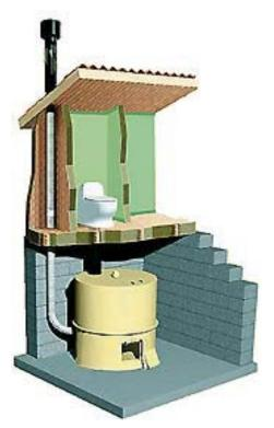
**Figure 3-7** Diagrams of the EcoTech Carousel composting toilet. (Adapted from EcoTech.)
