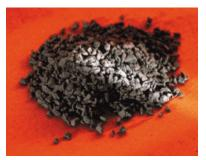
**Figure 6-4** Filtralite<sup>™</sup> aggregate media. (Adapted from Optiroc Group, Inc.)
