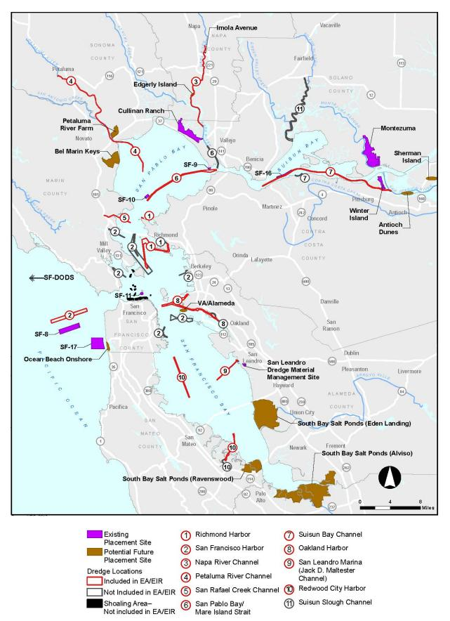
Figure 1. Federal Navigation Projects and Dredged Material Placement Sites
